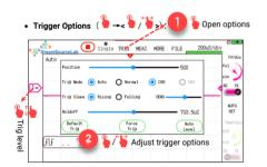
Trigger Sensitivity: Adjust the trigger level hysteresis window. Smaller values provide more sensitive triggering, while larger values increase stability in noisy signals.
